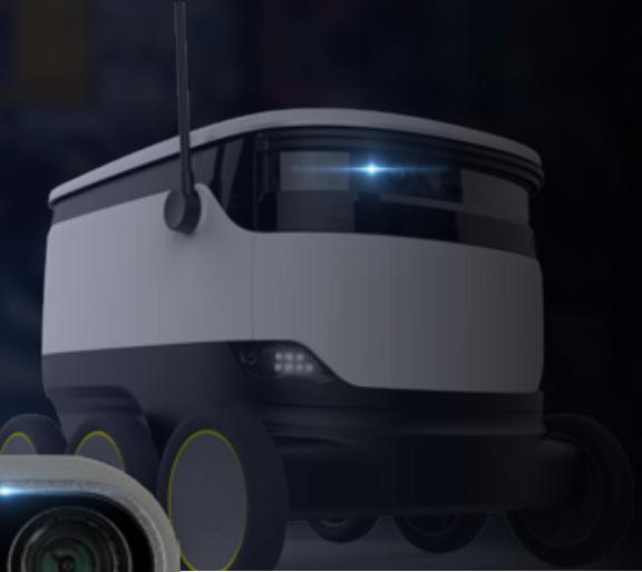
Designed around the NU4000 Robot-on-Chip (RoC), the M4.5S module integrates 3D sensing and image processing with AI capabilities, to provide robotic devices with human-like visual understanding. Integrating all robotic functions into a single processor enables simultaneous depth sensing and AI-based object detection and recognition, in a small, independent sensing module with optimal capabilities and superior performance.
